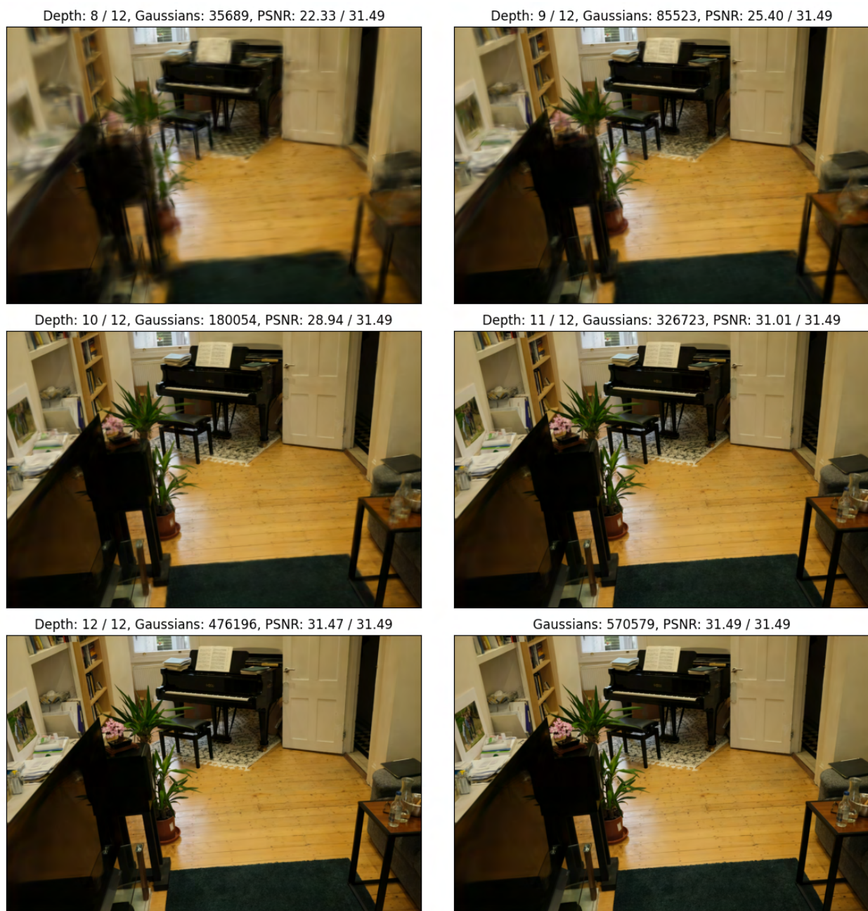
Figure C.3: Effect of depth variation on visual quality on room scene from Mip-NeRF 360 [2]. Using different levels of Octree results in changing granularity on images. Specifically, close points occur more blurry while far away points are less affected from averaging of Gaussian primitives.
