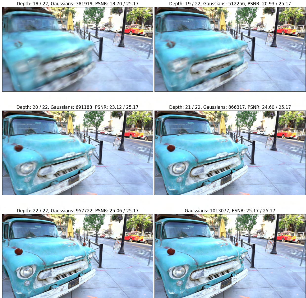
Figure C.2: Effect of depth variation on visual quality on truck scene from Tanks & Temples [19]. Using different levels of Octree results in changing granularity on images. Specifically, close points occur more blurry while far away points are less affected from averaging of Gaussian primitives.
