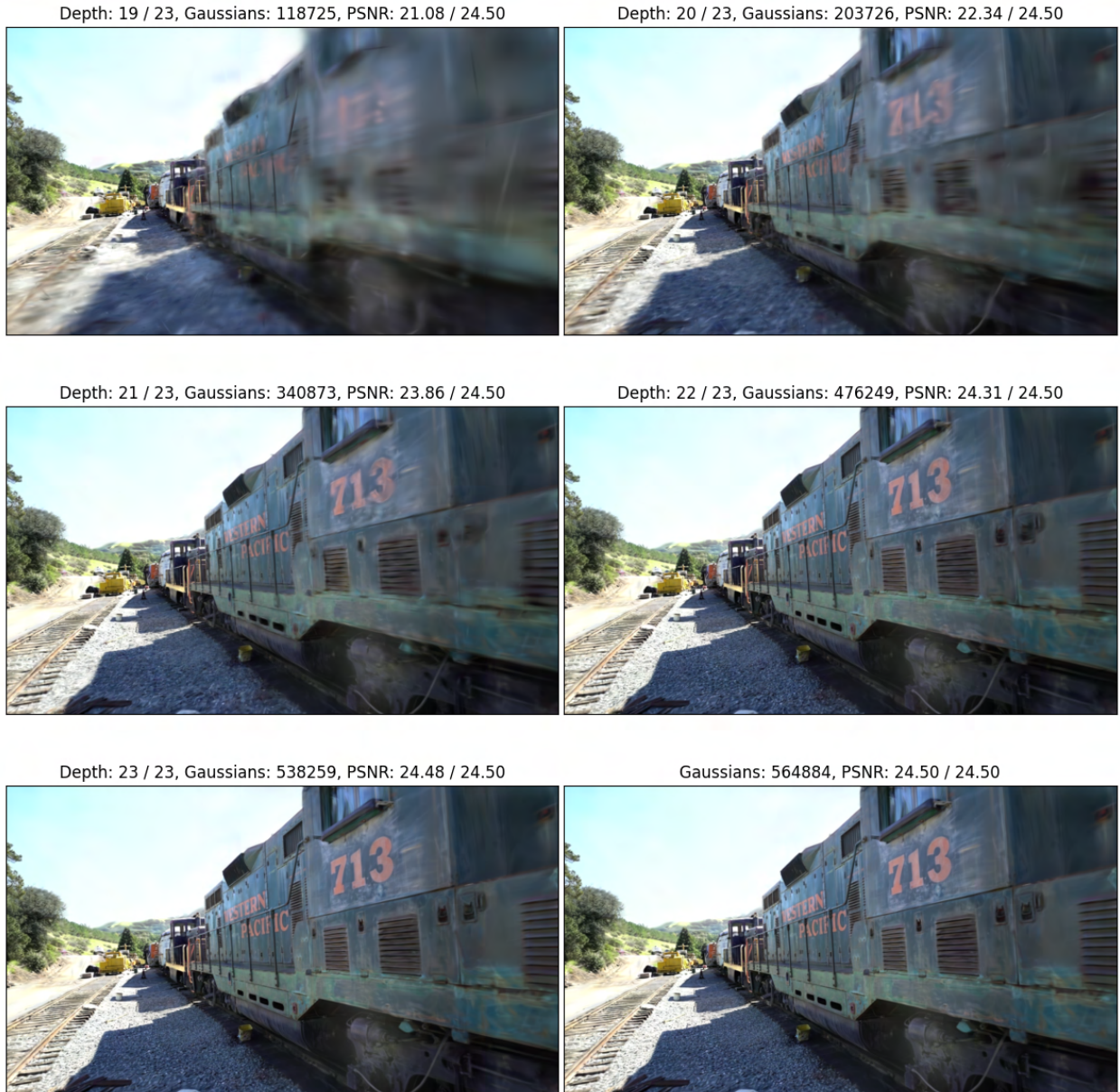
Figure C.1: Effect of depth variation on visual quality on train scene from Tanks & Temples [19] without compression. Using different levels of octree results in changing granularity of scenes. Specifically, close points occur more blurry while far away points are less affected from averaging of Gaussian primitives.
